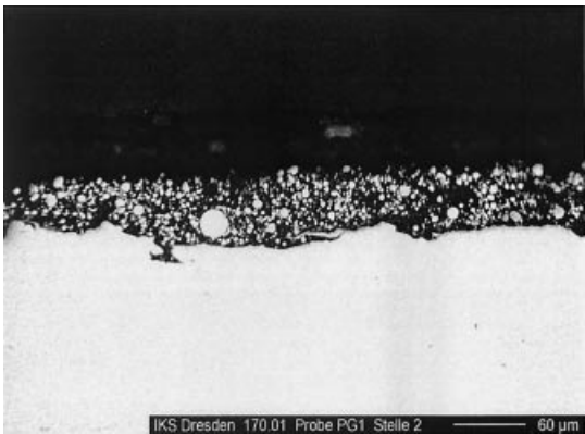
Figure 3. EP-zinc rich primer PUR-top coat
